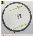
Undo the screws holding the gear tray, then lift the gear tray from the fitting
