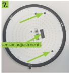
Secure the gear tray with its screws. Adjust sensor as shown on the next page.
