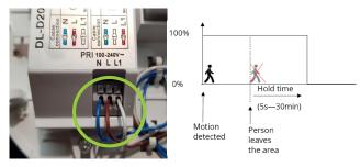
For 0% standby ensure blue wire is in "N" terminal, white wire in "L" terminal and brown wire in "L1" terminal.
