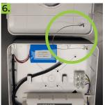
Ensure the cover connector cable is connected
